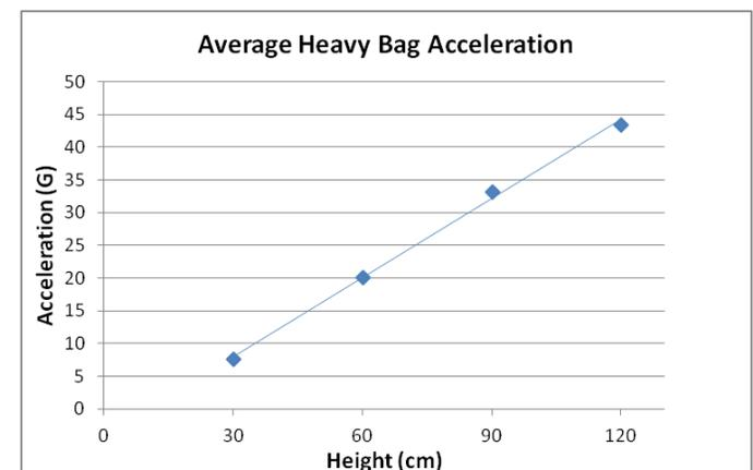
Figure 3: Heavy bag maximum impact acceleration vs. drop height.
